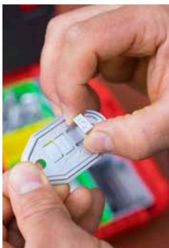
Second step: Click the pre-marked number inserts into the number plate.
